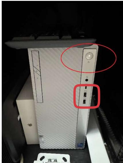
Power Light should be on. If light is not on Press one time to boot computer.
